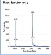
MALDI-TOF analysis of GMP-grade Recombinant Human IL-6 (Catalog # 206-GMP). The major peak corresponds to the calculated molecular mass, 20910 Da. The minor peak at 21127 Da is a matrixassociated artifact of the MALDI-TOF.
