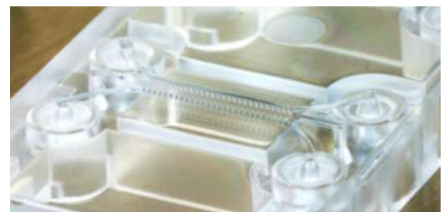
The underside of a microfluidic chip showing the size of its channels (250 microns deep). The chip is 25mm wide, measured from the edges shown above.
