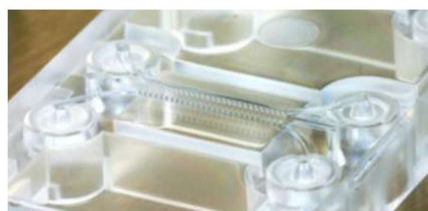
The underside of a microfluidic chip showing the size of its channels (250 microns deep). The chip is 25mm wide, measured from the edges shown above.
